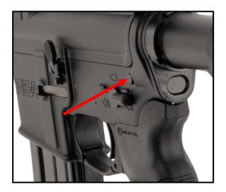
3. Pivot the lower receiver down and away from the upper receiver.
