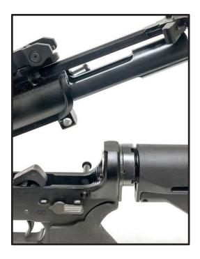
6. Remove the charging handle by pulling it backwards to the keyway and then down and out of the upper receiver.
