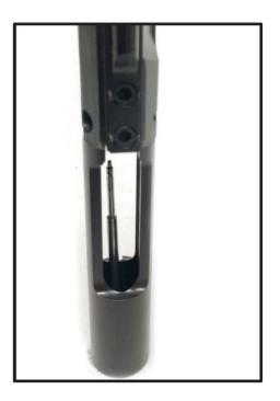
Push the bolt in toward the carrier until the bolt rotates and comes to a stop, then turn the bolt cam pin through 90° (i.e. at a right angle to its normal position).
