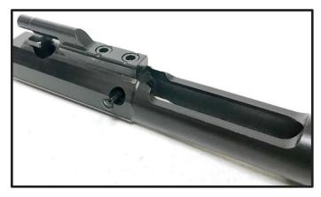
8. Tilt the bolt up and remove the firing pin.
